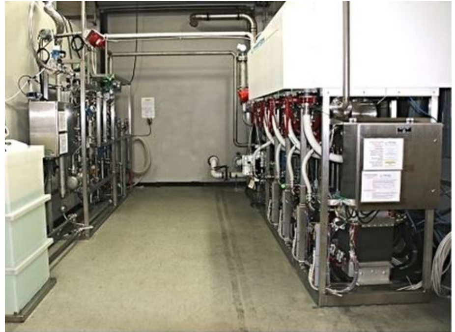
Pictured above: Proton OnSite's M Series megawatt platform, with the footprint of a 40' shipping container, is shown operating at more than 200 m 3 of hydrogen per hour. The modular design of the M Series enables solutions for an almost unlimited range of project sizes.
